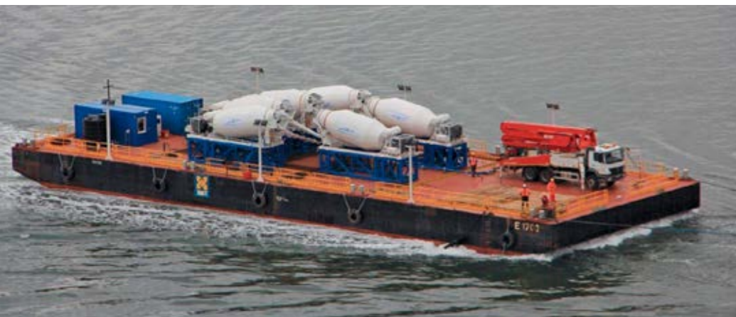
▲ The day passes...the concrete pump arrives: Concrete was poured around the clock for 15 days at the south pillar of the Firth of Forth bridge.
