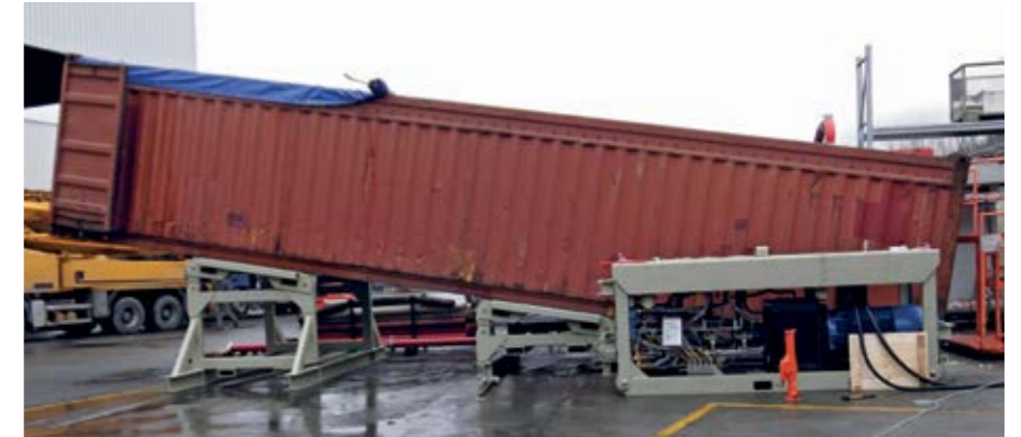
▲ The conditions at the planned operational site were simulated in the container positioned at a 10° slant.
