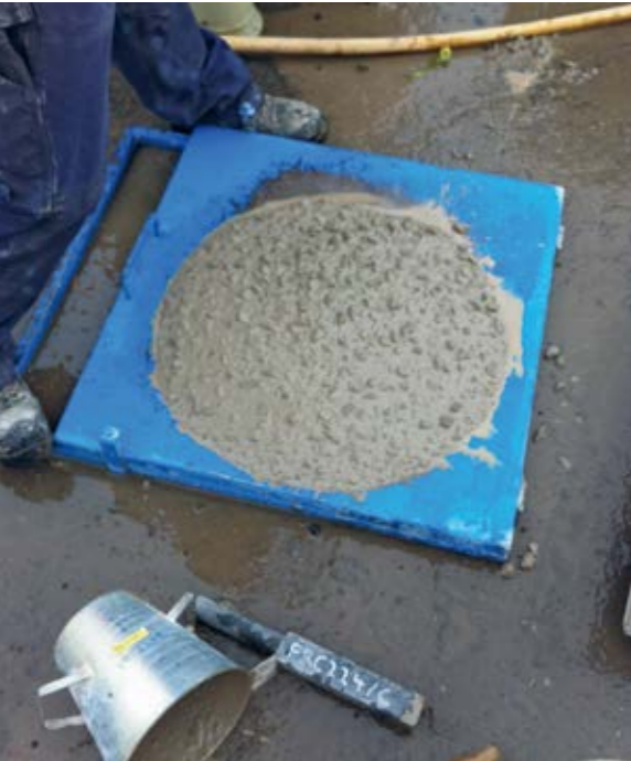
▲ Test of the flow consistency during the pumping tests: The pumpability of different types of concrete was determined.
