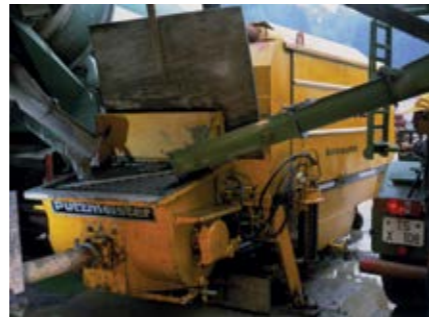
▲ World record 1989: 1,520 m at the Chiemsee tunnel using the TTS 14000
