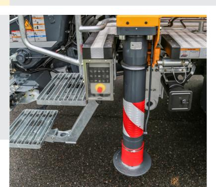
**Three defined support positions for the rear swinging support legs** Dimensions from the centre of the chassis: 1.70 m; 2.40 m; 3.30 m (fully flexible) **Four defined support positions for the front telescopic support legs**
