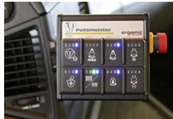
Above: The sturdy keypad has been fitted in an ergonomic position on the rear of the machine
