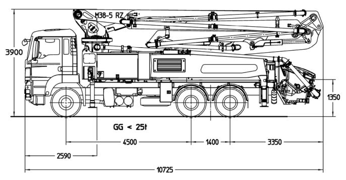
Note: Standard version. Dimensions and weights depend on truck, pump model and equipment. Dimensions in mm, MAN TGS 26.400.
