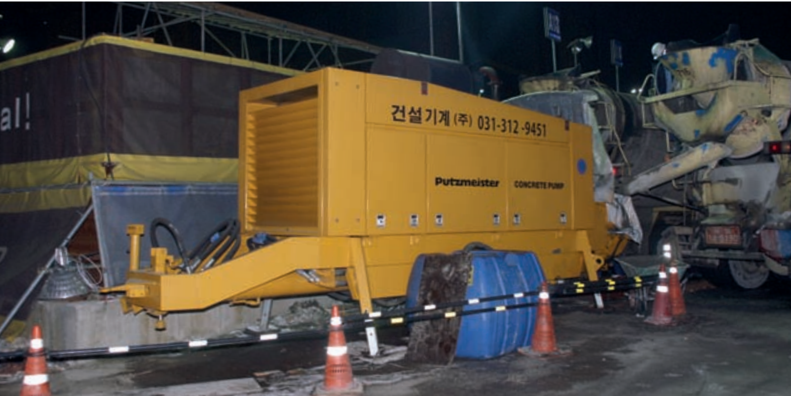
▲ A total of four BSA 14000 high pressure concrete pumps are in use – two HP-D and two SHP-D.
